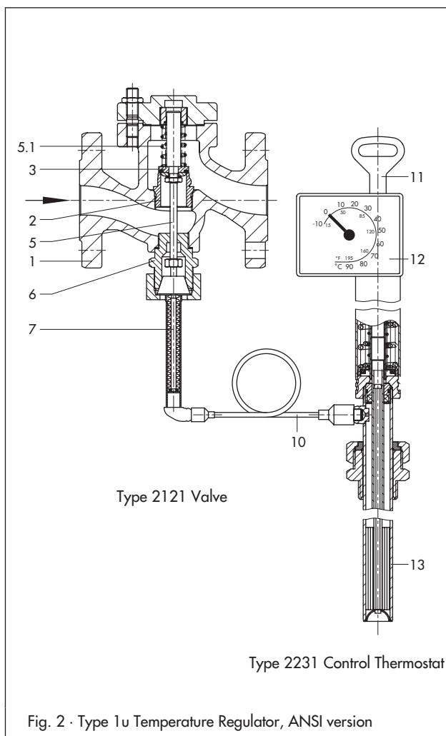
Fig. 2 · Type 1u Temperature Regulator, ANSI version
