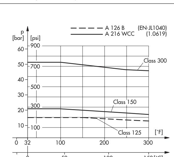
Specifications apply to the valve body.
