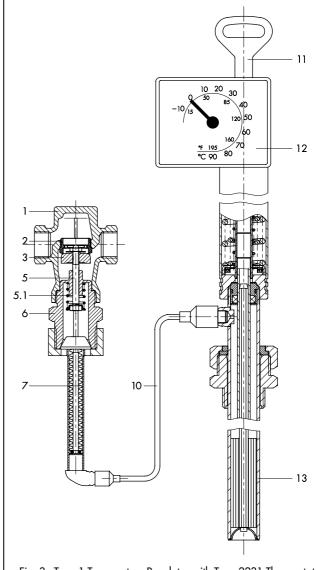
Fig. 3 · Type 1 Temperature Regulator with Type 2231 Thermostat
