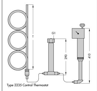
Fig. 6 · Dimensions of the thermostats with valves
