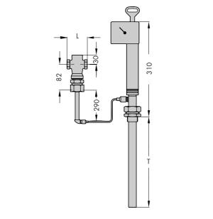
Type 1 Temperature Regulator with Type 2231/2233 Control Thermostat
